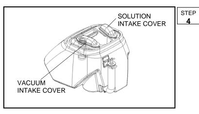
During operation, observe the following: The Admiral is equipped with clear internal covers to facilitate operator viewing of dirty solution and vacuum air flow
